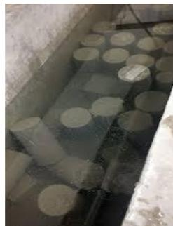
**Gambar 5.** Perawatan sample beton K 250
