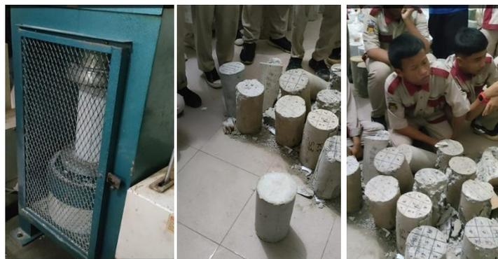
**Gambar 6.** Pengujian sample beton K 250
